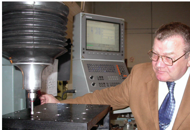
Marijan inspects the Jig Grinder (G32) he purchased and rebuilt himself in 2003. It's the most sophisticated and most accurate grinding machine owned by MTM.
